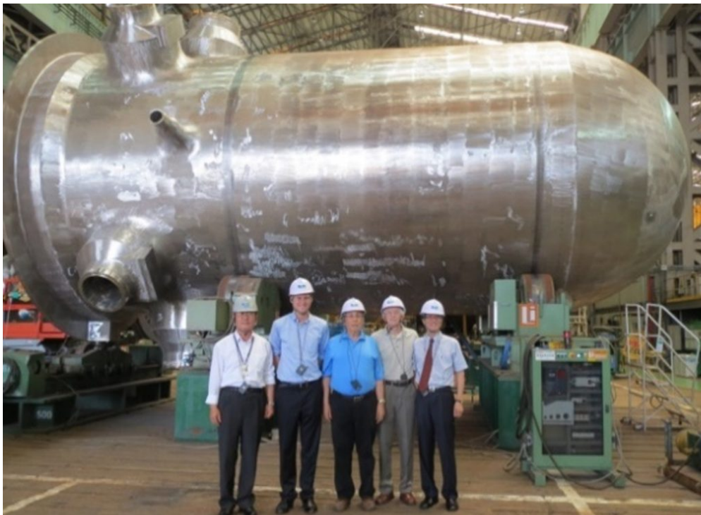
📷 South Korean manufactured reactor vessel intended for the Vogtle nuclear power plant in Georgia (USA). Source: Siegfried Hecker.
